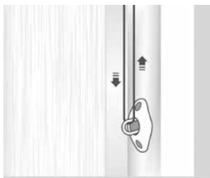
Cord Loop Tension device mountspull cord to window frame to prevent loose cords.
