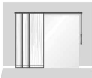
Reverse Stack Controls opposite of panel stack, left or right. Corded only.
